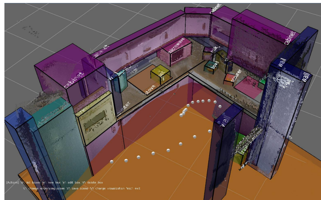
Fig. 1. Example of a kitchen reconstructed from a sequence of RGB-D observations within a robotic dataset. The appearing objects have been labeled (colored boxes). Gray spheres stand for RGB-D sensor poses.
