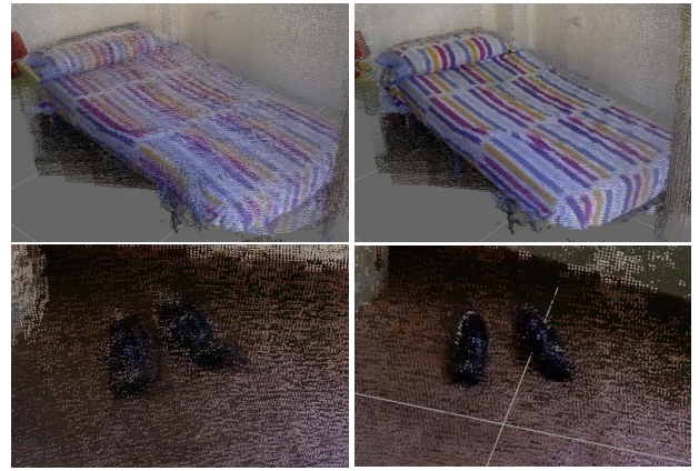
Fig. 4. Left, point clouds representing a bed-set and a pair of shoes reconstructed employing the sensor poses yielded by the robot localization. Right, the same objects reconstructed with the sensor poses refined with GICP.
