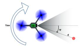
Fig. 8. The angle  $\psi$  is obtained with the centroid of the segmented color image that retains only pixels belonging to the beacon. Then,  $\psi$  is then used as error input for a PID controller that commands yaw in order reduce  $\psi$  to zero, effectively rotating the drone towards the beacon.
