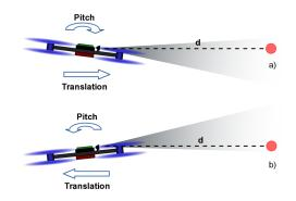
Fig. 9. Distance PID controller response. a) Current distance "d" is greater than target distance, the drone approaches by changing its pitch towards the beacon. b) Current distance "d" is smaller than target distance, the drone retreats by changing its pitch away from the beacon.
