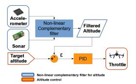
Fig. 6. Blue: non-linear complementary filter [20] for altitude that integrates twice the accelerometer data to obtain the current altitude and eliminates accumulative the bias using the data from the sonar. Orange: PID controller for altitude that commands the drone's throttle.
