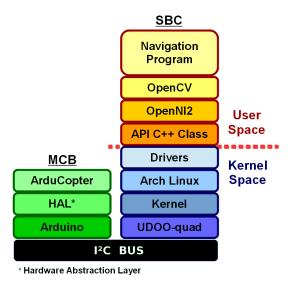
Fig. 5. Software hierarchy. The left stack is for the Multicopter Control Board. The right stack for the Single-Board Computer, which runs linux and is divided into kernel and user space.
