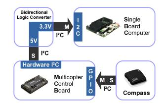
Fig. 4. Communications between the SBC and the MCB. The MCB uses a native  $I^2C$  bus to communicate with the SBC, and a software simulated  $I^2C$  with GPIO pins for the electronic compass. M denotes Master of the bus and S denotes Slave
