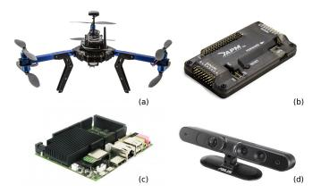
Fig. 3. Some of the employed hardware. (a) RTF-Y6 Hexacopter. (b) APM-2.6 Multicopter Control Board. (c) UDOO-quad 4 core 1GHz ARM development board. (d) Asus Xtion PRO live RGBD camera.
