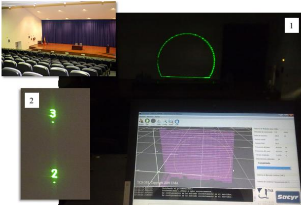
Figure 5: TCS operation example. The TCS system scans the screen of an auditorium, generates a triangular mesh from the surveyed points (see the user interface on the bottom-right of the figure), and intersects the mesh with a simulated planned tunnel. Finally, (1) the resulting profile is projected on the front. During the TCS operation, (2) any desired text can be also projected on the excavation wall.
