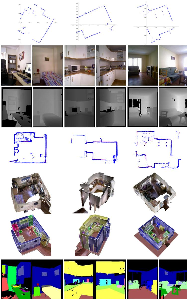
**Figure 4.4:** Excerpts of information provided by Robot@Home. From top to bottom, examples of 2D laser scans, RGB images, depth images, 2D geometric maps, reconstructed rooms, labeled reconstructed rooms, and labeled depth information. Taken from [123].
