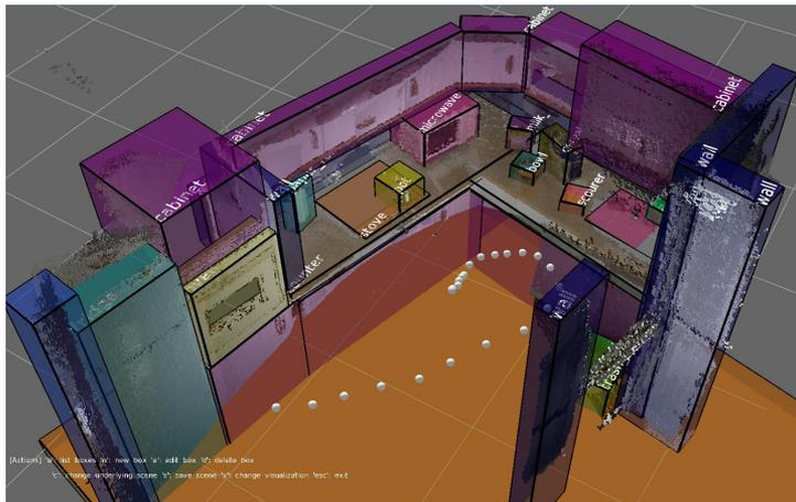
**Figure E.1:** Example of a kitchen reconstructed from a sequence of RGB-D observations within a robotic dataset. The appearing objects have been labeled (colored boxes). Gray spheres stand for RGB-D sensor poses.
