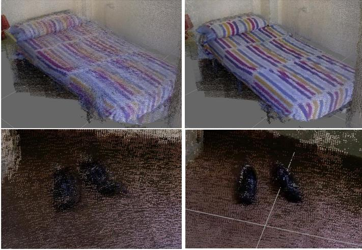
**Figure E.4:** Left, point clouds representing a bed-set and a pair of shoes reconstructed employing the sensor poses yielded by the robot localization. Right, the same objects reconstructed with the sensor poses refined with GICP.
