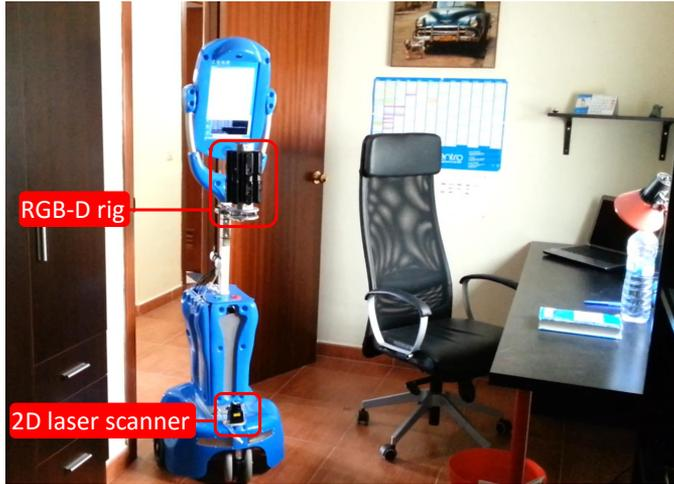
**Figure F.7:** Robotic platform used to collect the Robot@Home dataset.
