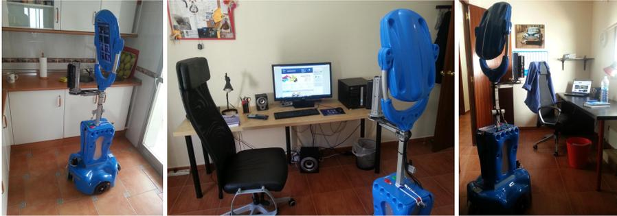
**Figure 4.3:** Giraff robot while collecting sensory information. The basic robotic platform was endowed with a rig of 4 RGB-D sensors mounted on the *robot's neck*, and a 2D laser scanner on its base.
