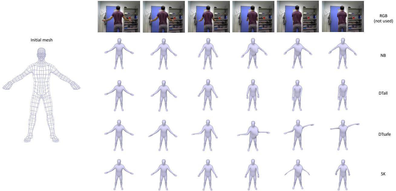
Figure 1. Results after running the optimization problem to align a given initial mesh of a person with geometric data associated to different postures. The first tested images (left columns) observe a person whose posture is close to the initial mesh while the person’s posture in the the last ones (right columns) is considerably different from that of the initial mesh.
