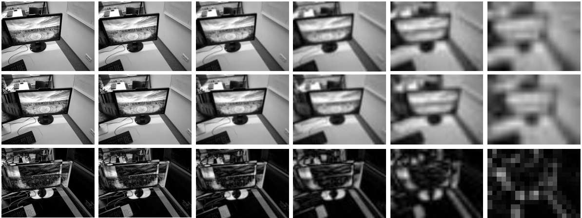
Figure 3.1: Example of an image pyramid. Resolution goes from VGA (left) to 15 \times 20 (right). The first rows show two consecutive intensity images taken with an RGB-D camera, and the last row shows the residual image (absolute difference between the two). It can be observed that the misaligned areas cover many pixels in the original images, whereas they are only one or two pixels wide in the coarsest image. Hence, any linearization applied on the finest level would not help to align both images while the same process applied on the coarsest level would work (but not with precision).
