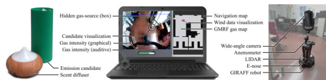
Figure 8: (left) Ultrasonic scent-diffuser and one of the gas source candidates. (middle) User interface for teleoperating the robot running on a laptop. (right) Giraff telepresence-robot equipped with an e-nose and an anemometer for remote sensing, and a LIDAR for self-localization.
