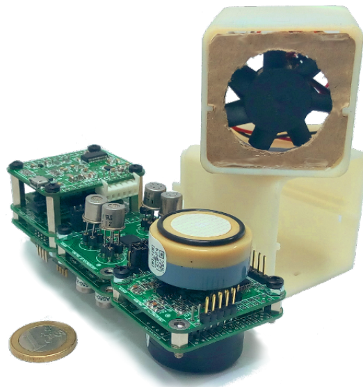
Figure 1. Picture of the e-nose prototype built for the IRO project. Its modular and compact design allows it to be easily mounted on a mobile robot and adapted to the application requirements.
