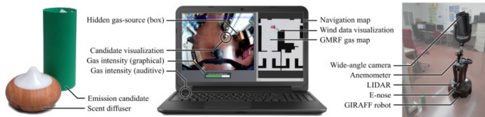
Figure 10. (Left) Ultrasonic scent-diffuser and one of the gas source candidates. (Middle) User interface for teleoperating the robot running on a laptop. (Right) Giraff telepresence-robot equipped with an e-nose and an anemometer for remote sensing, and a LIDAR for self-localization.
