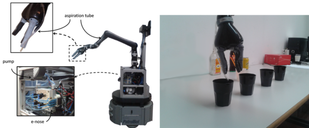
Figure 4. The Rhodon robot with the robotic arm used in the experiments.
