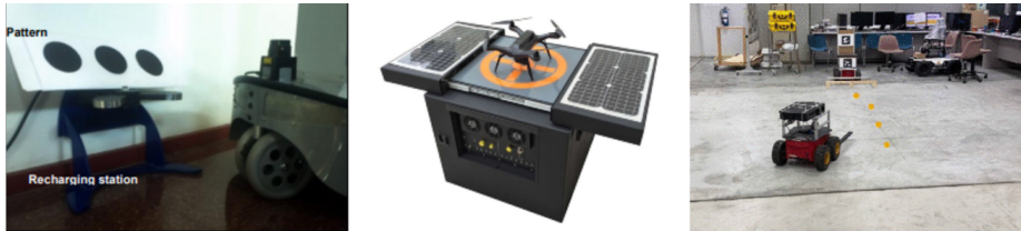
Fig. 1. Left, charging station for a domestic robot composed of three circles [4]. Middle, station for a drone consisting of a circle with a cross [11]. Right, a charging station identified by two QR codes [5].
