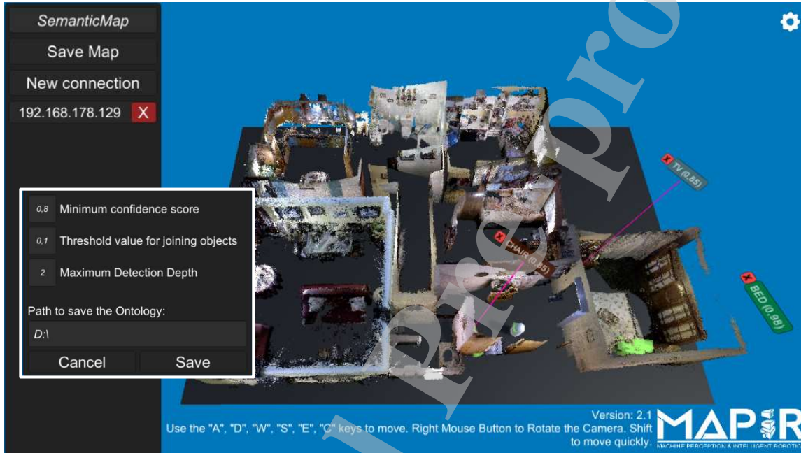
Figure 4: Graphical User Interface designed to support human-robot interaction including buttons, text fields, and a visualization of the virtual environment with different mechanisms for its modification. Down left, a screenshot of the floating window permitting an advanced configuration of the system.
