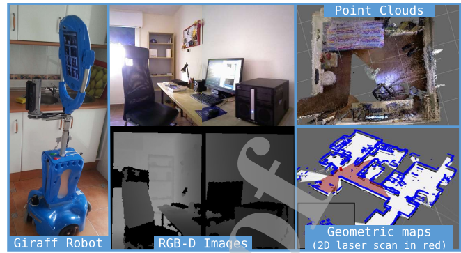
Figure 7: Mobile robot used to collect the Robot@Home dataset along with some samples of the data it provides.
