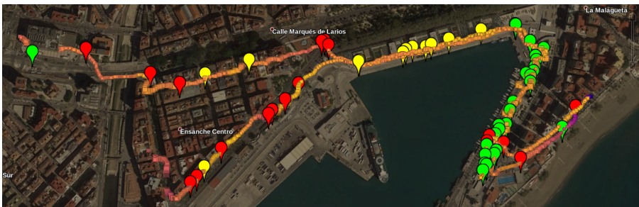
Figure 6.3: Simple smell map of Malaga’s port and sea promenade created with our e-nose and a GPS-enabled smartphone. The colored markers show locations where training data was taken, whereas the colored path shows automatically generated smell labels. In this case, both the training data and output are for the same general area, but once trained, the e-nose can also recognize smells in new places or provide information to a robot for tasks like GSL or GDM.
