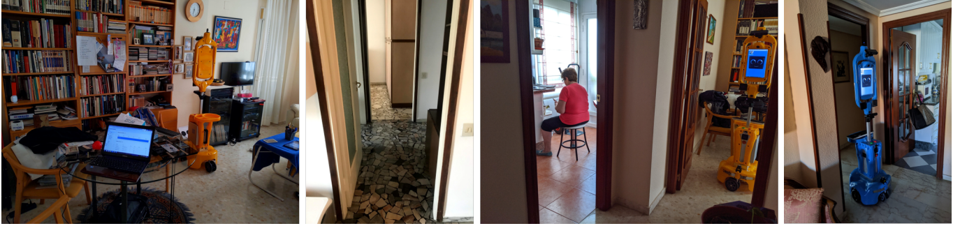
Figure 4: Pictures of different apartments where the Giraff-X robot was installed. As can be seen, different flooring types, cluttered areas, and narrow doorways are common in these environments, making autonomous navigation a challenging task.
